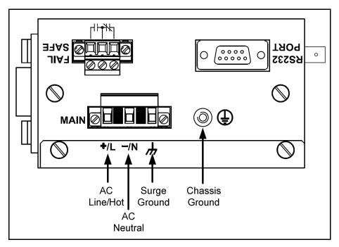
Figure 4 - RS910L Power Supply Inputs
